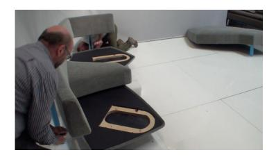
Slide the base (1) over the mounting plates of the back supports (2).
